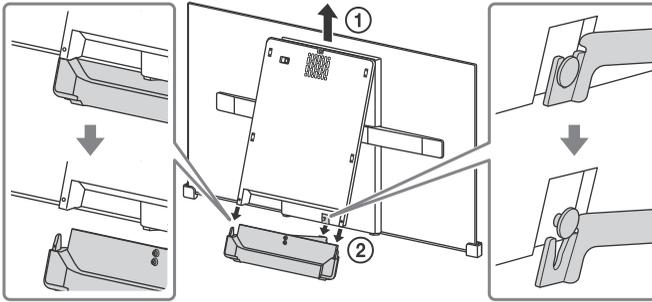
**5** Close the center block by releasing the hinge lock.
