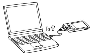
The player's battery is recharged while the player is connected to a running computer.
